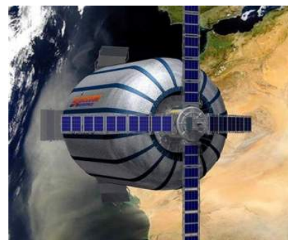
Figure 8 -Genesis, created by Bigelow Aerospace, is one of the successful uses of inflatable structures in space. The inflatable design used to make this was initially developed by NASA's TransHab Project.
