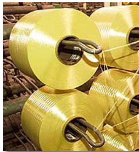
Figure 10 - Spools of Kevlar 29 (the same material used for bullet proof vests) will provide some level of protection against micrometeorites.
