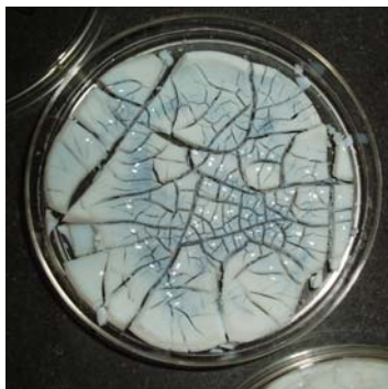
Figure 6 The cracking pattern in a dried 0.5 M sol-gel sample.
