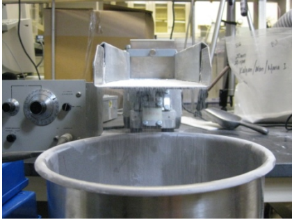
Figure 6: Picture of the charge density apparatus.
