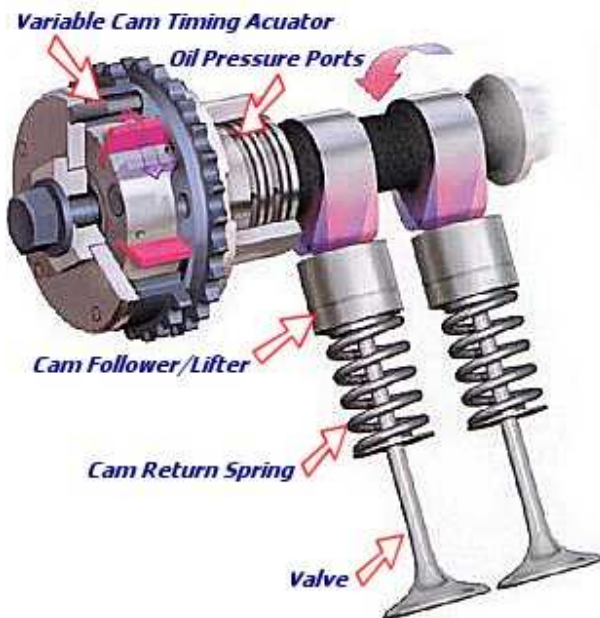
Fig. 2.2.1 – Camshaft – forces intake and exhaust valves down using egg-shaped lobes [11]
