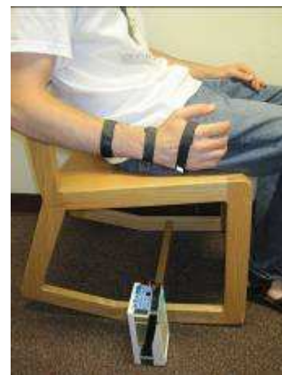
Figure 4. The orientation of the wiimote and the user’s arm when in a sitting position.
