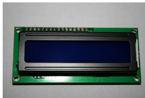
Figure 5: The LCD screen has a number of contact points (top left). They are connected to input digital pins, 5V and ground. It is a 16x2 LCD module.
