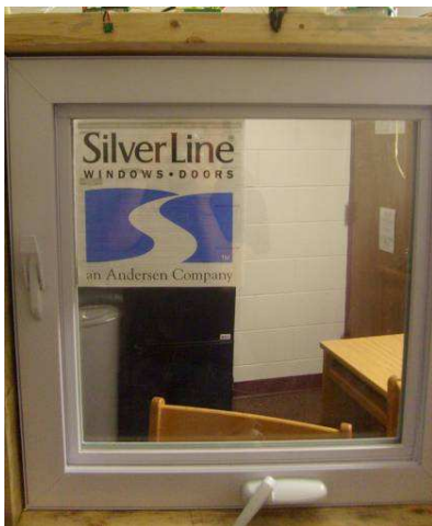
Figure 1: The casement window we used for our project. Has a crank to turn the window to make for easy opening.
